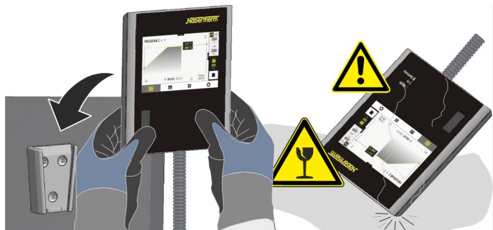
Fig. 71: Place the controller in the holder on the furnace (similar to the picture)
