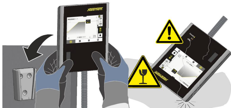
Fig. 55: Place the controller in the holder on the furnace (similar to the picture)
