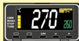
Example of an over-temperature limiter
