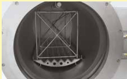
Charging support and TUS measuring frame for retort furnace NR 20/11
