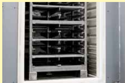
Charging trolley for chamber furnace N 2200
