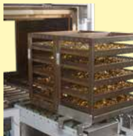
Continuous furnace for bulk materials in baskets
