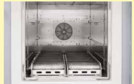
Roller conveyor in furnace chamber
