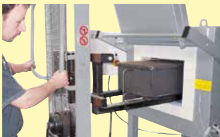
Working with protective gas boxes for a protective gas atmosphere using a charging cart
