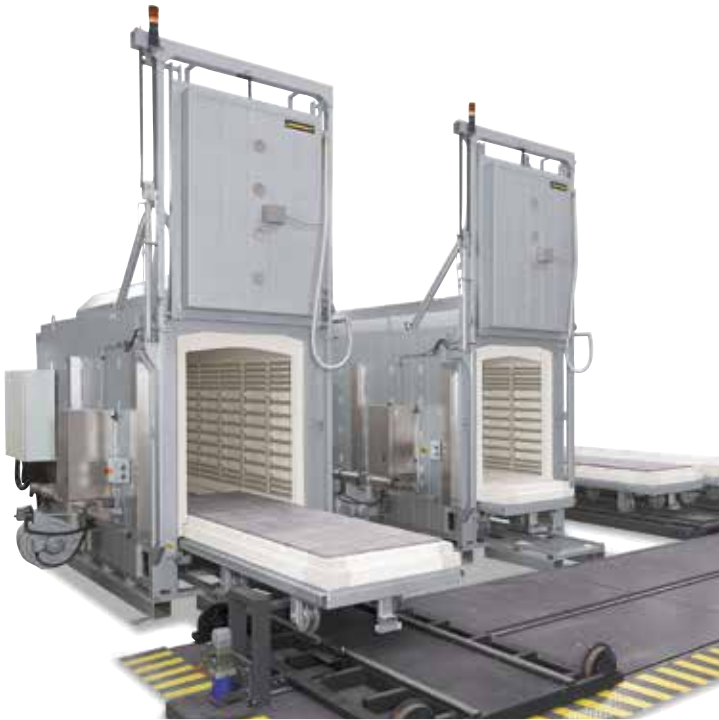
Combi furnace system consisting of two bogie hearth furnaces W 5000/H and two additional bogies incl. bogie transfer system and incl. necessary park rails
