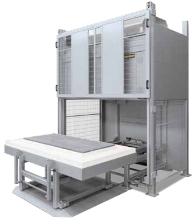
Bottom loading furnace HF 1220/LBS with fiber insulation, safety barrier to safeguard the danger zone and manually movable table for ease of loading and unloading
