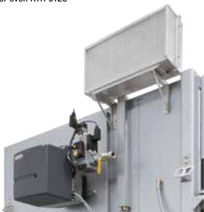
Direct gas-firing at a chamber oven
