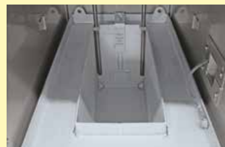
Crucible made of high-quality CrNi steel
