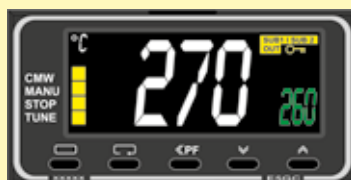
Example of an over-temperature limiter
