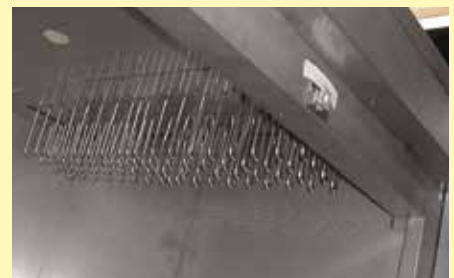
Enclosed heater coils on electrically heated models
