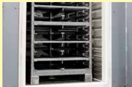
Charging trolley for chamber furnace N 2200
