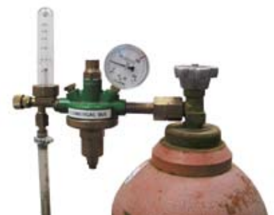
Pressure reducing valve with assembled flow meter
