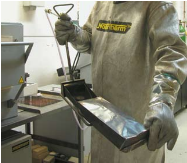
Protective gas annealing bag in operation
