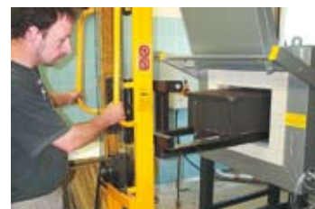
Winch stacker with hardening box and furnace
