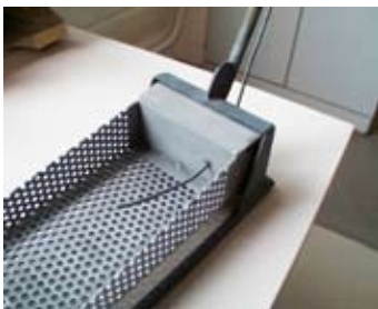
Thermocouple integrated in holder
