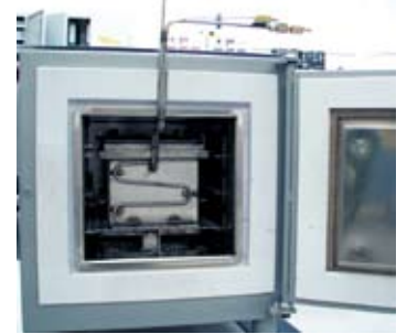
Air circulation furnace with protective gas box
