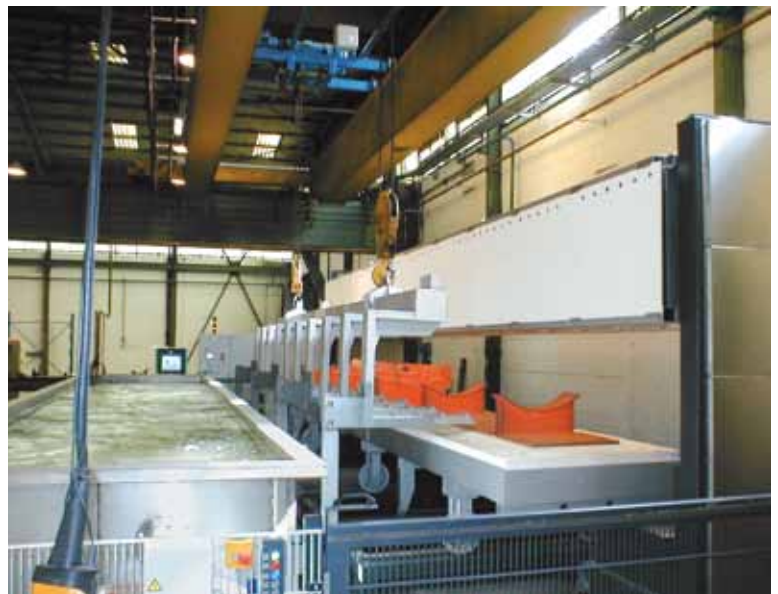
Manual heat treatment system for hardening of steel rods see page 62/63
